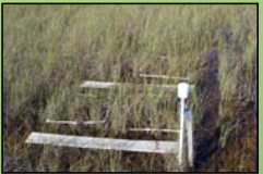
Figure 5. Cladium plots at LC with an Infinities Acoustic water level gauge.
