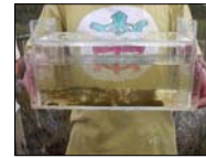
Figure 5. Flocculator partially filled with floc
